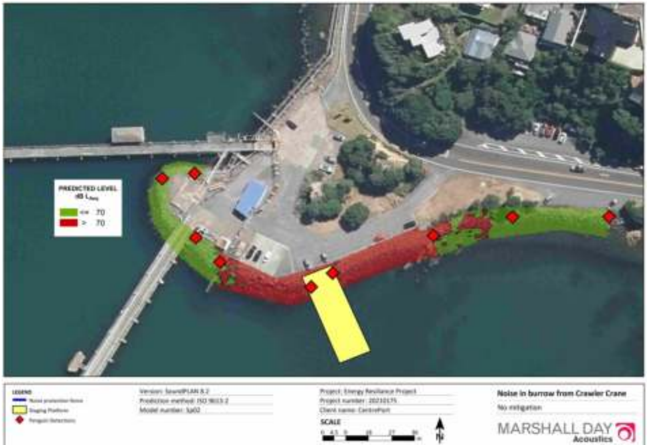
Figure 2. Unmitigated predicted noise levels received inside kororā burrows (assuming a 5 dB reduction compared to noise in the air outside) from crawler crane movements.
